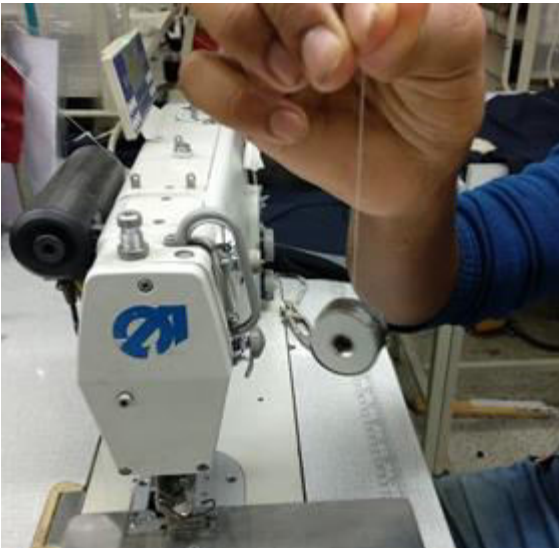
Setting up of Correct Thread Tension
